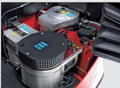
Ex-protected drive/steering/lift motor and hydraulic tank
